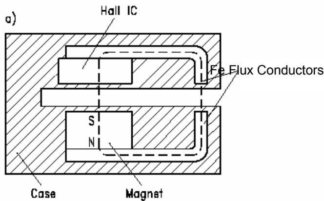
a) Magnetic flux through the Hall-effect switch with no vane in the gap
