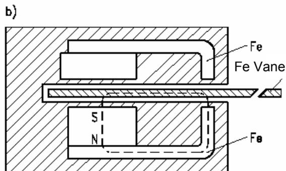
b) Magnetic flux short-circuited by the soft-iron vane
